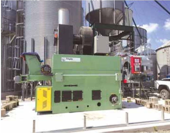
One of the attractive features of the BioDryAir systems is that they can be installed as a parallel heat source on an existing dryer. The operator simply switches the hot air input from the gas-fired burner to the biomass system or back as needed.
