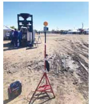
The Pit Stop is an LED light operated from a sensor and reflective strip on a trailer to help with unloading.
