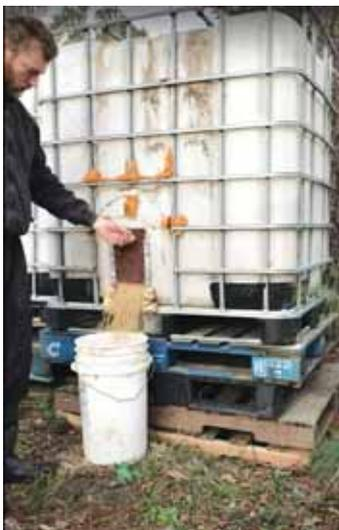
**A used IBC tote with the top cut off and a small sliding door added to the bottom stores bulk feed and can be moved with pallet forks.**
