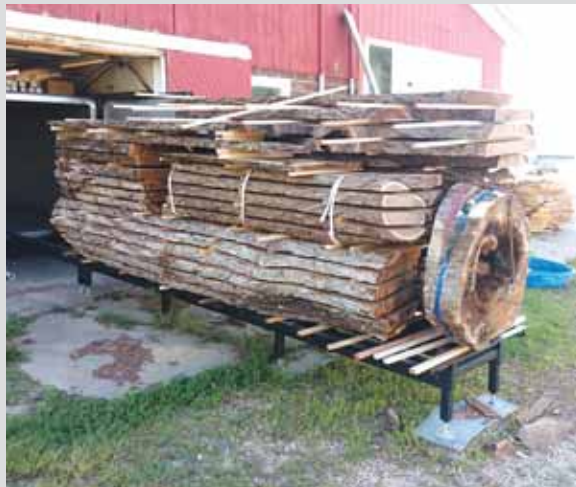
Manske saves out large edge slabs and dries them with his vacuum kiln.
