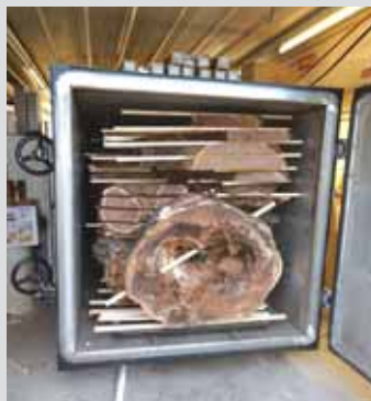
The iDry 2.0 Vacuum Kiln can hold up to 2,000 board feet.
