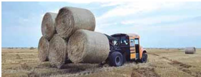
Henry eliminated the center bale spear and just uses two after finding that the center spear couldn't penetrate corn stalk bales.
