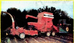
The Koepke-built combine features a 729A Uni-Sheller mounted on a trailer. Power for the combine, and the trailing chopper, comes from the tractor's 1,000 rpm pto.
