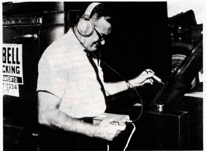
By holding Motorprobe's snout against a moving part, you can hear trouble spots before serious damage occurs.
