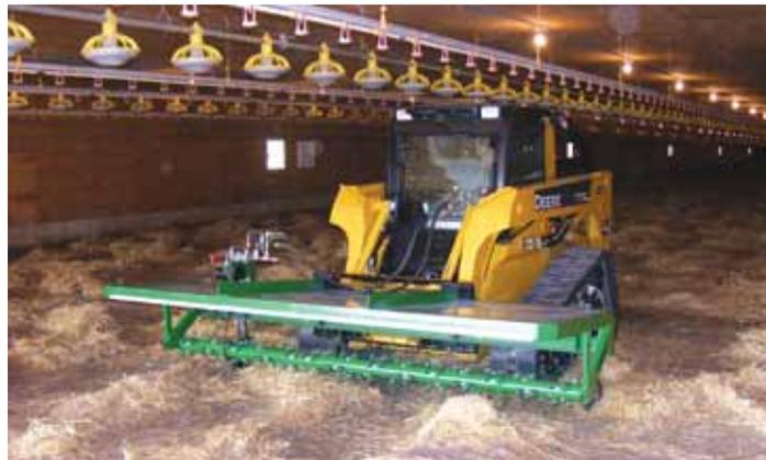
Rotary fork spreads clumps and bales of straw or shavings to create a uniform bed.
