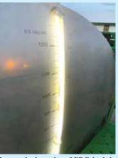
Inexpensive low voltage LED lights help to light up the water gauge on a sprayer
