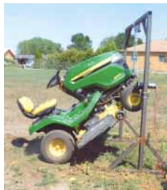
Greg Waldie's lift is made from 2-in square tubing and uses an ATV winch to lift a mower for repair work.
