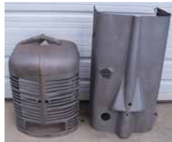
Before and after photos show the results of using Chlor*Rid salt remover after sand blasting and before painting. Paint contractor Jim Deardorff says his system can remove rust from 10-gauge metal without affecting the metal.
