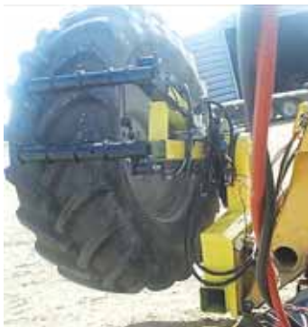
Tire Wrangler can be mounted on a skid steer, loader or forklift and can even handle 2,000 lb. floater tires.
