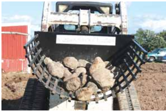
Rock Master showing reinforced steel bars with slightly longer center bars to keep bucket centered.
