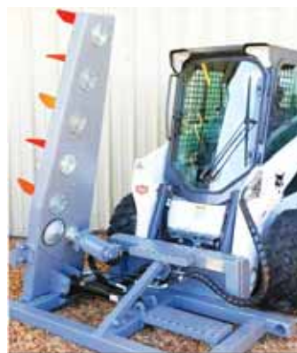
Hydraulically-driven vertical blades on an HMI Bed Buster mount on a skid steer to fluff up sand or compost materials in free stall barns.
