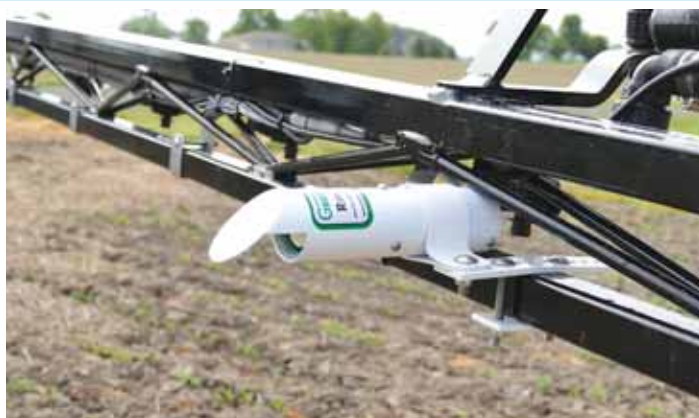
A Greentronics sonar unit is used to control boom height on a field sprayer.
