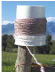
The bucket rests over the top of a fence post and can freely turn to feed wire.
