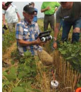
Soil health is monitored through CO<sub>2</sub> levels using the Soil Talker field testing device.
