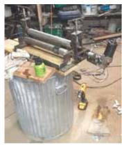
Bruhn made his metal bender using a wiper motor and rollers welded to angle iron.
