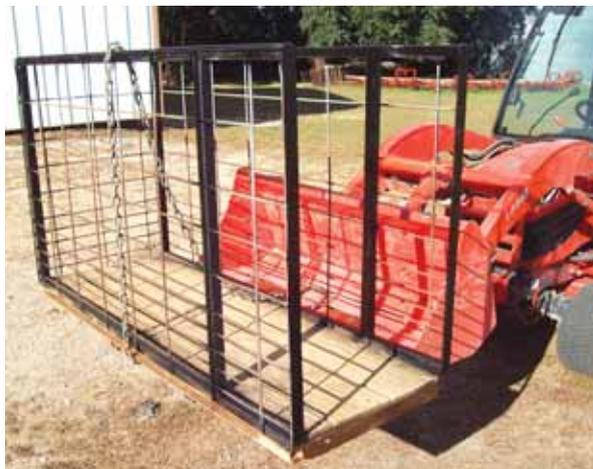
Safety cage base is designed to slip over the lip of the bucket and works on different size buckets.
