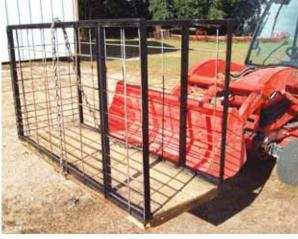
Safety cage base is designed to slip over the lip of the bucket and works on different size buckets.
