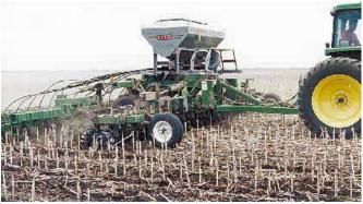
Hiniker air seeder unit mounts on Rawson coulter cart ahead of modified Max-Emerge planter.
