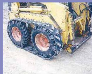
Tracks are made from used rear tractor tires. Steel guides bolt to each side of track at 8-in. intervals.
