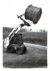
"My grapple fork is also a materials handling dream. I can use a 4-ft. long chain in front of the arms to haul 8 by 10-ft. sheets of steel. By mounting another steel frame on the fork I can use it as a light crane to lift materials such as 150-lb. rafters 18 ft. high."
