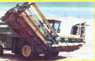
A Deere 24 ft. header was cut down to 20 ft. for center section. Two other used Deere headers were "retooled" to make the 10 ft. folding wings. Sickles overlap so there's no "cutting gap" between the three sections.
