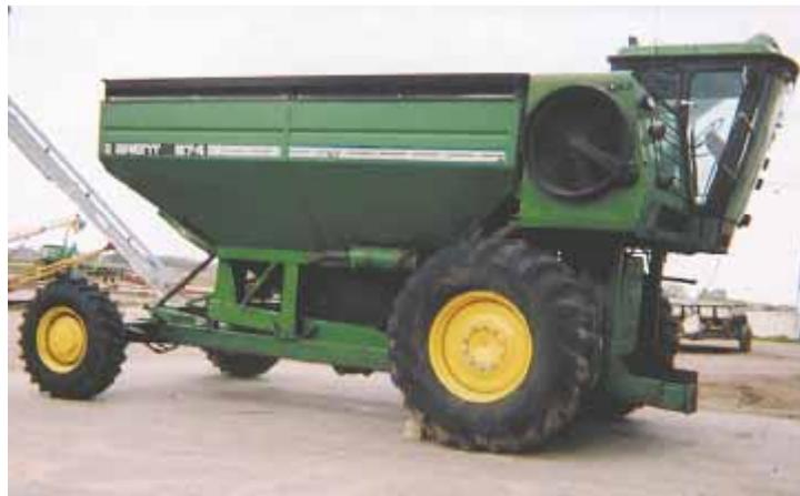
To make this self-propelled grain hauler Harlan Schlaak combined a Deere 8820 combine with a 674 Brent grain cart.
