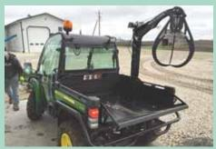
UTV-Mounted Rock Hawk is designed to pick up rocks in the field and then swing them over into a steel replacement box.
