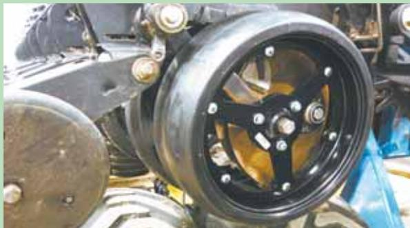
Mudsmith has reinvented the gauge wheel with an all-new design that cleans itself.
