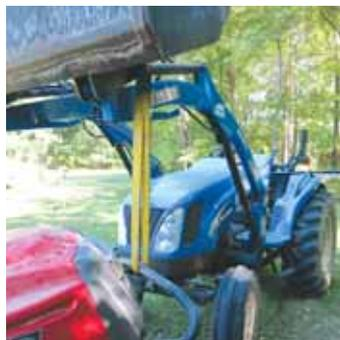
Bucket-mounted, sewn loop end strap shown above hooks onto the push bar on Willett's riding mower, lifting it for service work.
