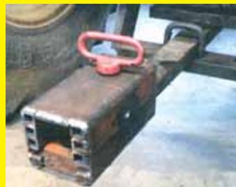
My homemade hitch adapter lets me quickly convert my tractor's drawbar to a multi-ball hitch. It's designed so the multi-ball hitch slips inside a short length of
