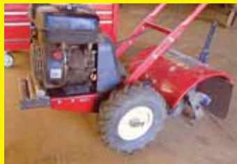
My brother-in-law bought this rototiller for \$40 but it was a real "arm stretcher" because of the way it would bounce around while tilling. After trying it out myself, I went to my shop and made a "weight box" for the front end. I just kept welding on heavy pieces of steel shafting until I got it to the point where I could walk alongside the tiller and run it with one hand. Smooth and steady. (Jim Lacey, 47582 240<sup>th</sup> St., Dell Rapids, S.Dak. 57022)
