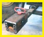
My homemade hitch adapter lets me quickly convert my tractor's drawbar to a multi-ball hitch. It's designed so the multiball hitch slips inside a short length of
