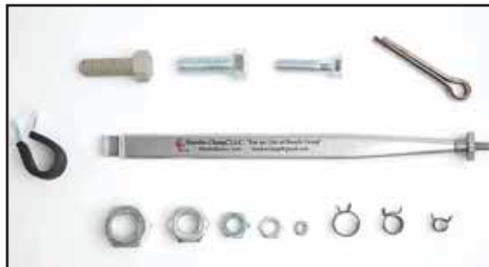
Handee Clamp has a sliding “jaw” on one end and an adjustable nut on the other end. You slide jaw out and place a nut or bolt on it, then tighten nut to lock jaw in place.
