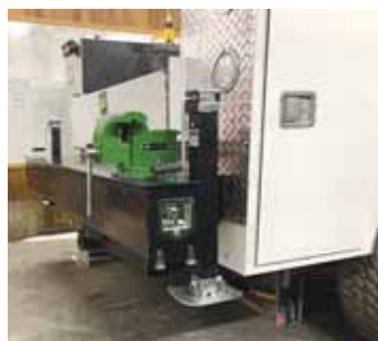
Outrigger jack stands on both ends of workbench help keep truck stable.
