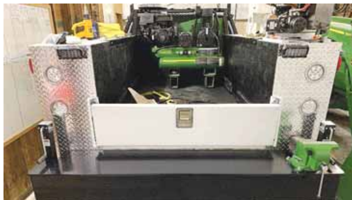
Home-built workbench measures 14 in. deep and stands more than 1 ft. taller than the small factory bumper it replaced.
