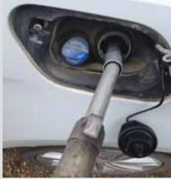
**Fritz Groszkruger, Dumont, Iowa:** "Our 2015 VW Golf TDI diesel has a feature that prevents you from making a mistake and putting gas into it. When we started storing diesel in a tank that used to hold gas, I had to find a way to fuel up the TDI. So I cut off a piece of an old BBQ axle, which fits into the fuel opening. Works just fine."
