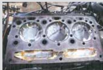
**Joe Johnson, Meridian, Miss.:** "I was working on a 3-cyl. Perkins diesel engine from a Massey Ferguson 150. I needed a way to keep debris from falling into the cylinder bores when cleaning the engine block surface for head gasket replacement."
