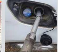
Fritz Groszkruger, Dumont, Iowa: "Our 2015 VW Golf TDI diesel has a feature that prevents you from making a mistake and putting gas into it. When we started storing diesel in a tank that used to hold gas, I had to find a way to fuel up the TDI. So I cut off a piece of an old BBQ axle, which fits into the fuel opening. Works just fine."
