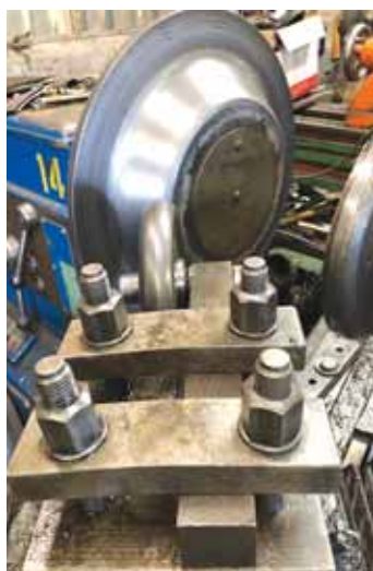
Metal spinning involves attaching a flat circular metal disk to a lathe and pressing a die against it. As the metal spins it starts to change shape, thinning and expanding where pressed.
