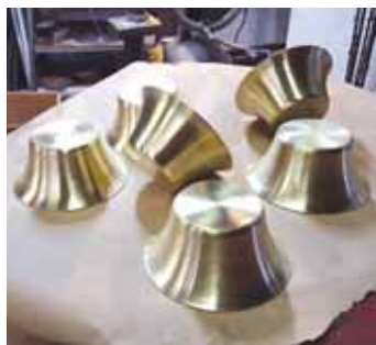
Metal spinning involves attaching a flat circular metal disk to a lathe and pressing a die against it. As the metal spins it starts to change shape, thinning and expanding where pressed.
