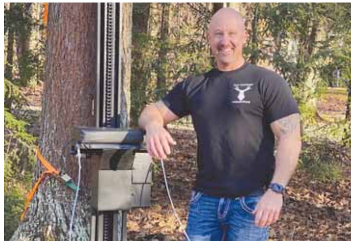
Battery-powered Tree Runner stand moves up and down on a cogged trolley. “It can be moved up or down to change positions for a better view,” says inventor Shawn Booth.
