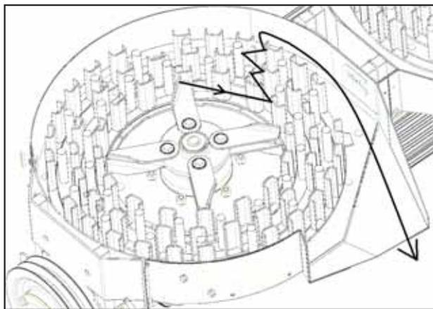
Seeds and chaff enter 2 side-by-side impact mills composed of a rotor and stator. Center fan blades accelerate seed entering each mill against U-shaped stator elements (top). The 2 mills spin in opposite directions, discharging material into the straw stream.
