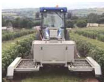
RootWave technology uses electricity to kill weeds. The company offers a handheld weeder and is working on a tractor-powered machine.
