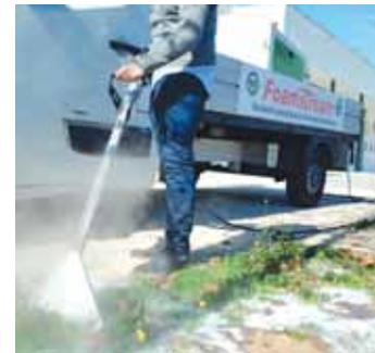
Foamstream combines hot water with a biodegradable foam applied by a wand. Hot water kills the plant matter, and the foam insulation keeps the heat working longer.
