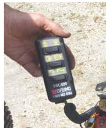
Lifting device is operated with a handheld control.
