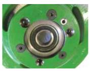
Elevator drive shear hub replaces the OEM hub with a 5-min. bolt replacement.
