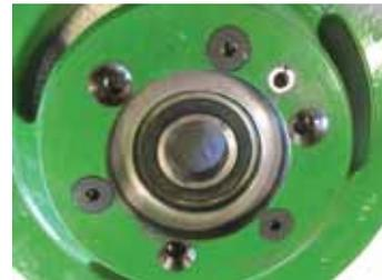
Elevator drive shear hub replaces the OEM hub with a 5-min. bolt replacement.
