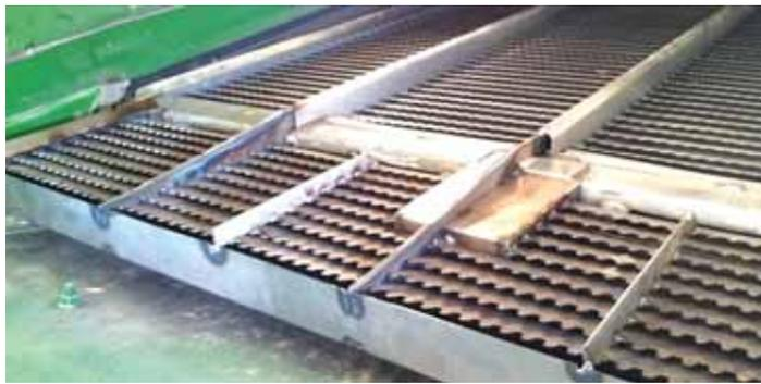
Sieve extension for Deere S-series combines greatly reduces the load on the return system.
