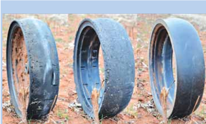
Photo shows OEM gauge wheel (far left) and urethane wheel (center) after 146 acres of use. New 4Ag wheel at far right has 1,233 acres on it.
