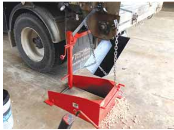
Gravel is augered into bottomless 3-sided drag box, which hangs from back end of gravel truck.
