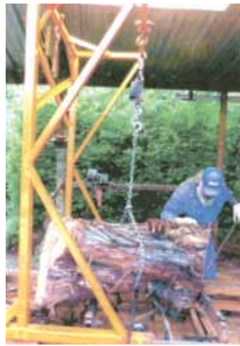
Cradle lift can easily lift short, heavy logs onto sawmill bunk (left). It rides on 4 small wheels and rolls back and forth on the same tracks as the sawmill.
