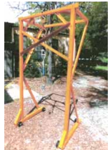
Cradle lift can easily lift short, heavy logs onto sawmill bunk (left). It rides on 4 small wheels and rolls back and forth on the same tracks as the sawmill.
