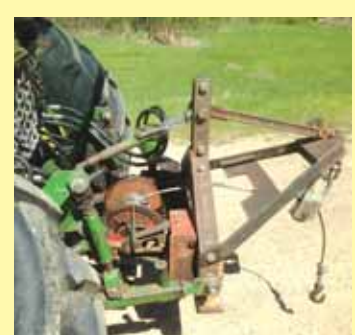
Arch’s electric winch is used to pull logs out of the woods.
