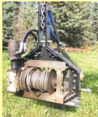
Rhoades used the cross braces off an old plow frame to build this 3-pt. mounted logging arch equipped with a triangle-shaped boom.
