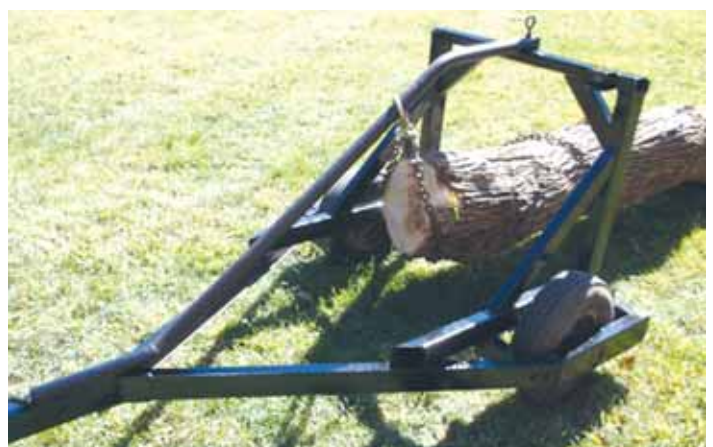
Petrevich wraps chain around log and attaches it to hook on skidder’s slider bar. “As I pull forward, the log will raise itself and automatically drop to the ground when I stop,” he says.
