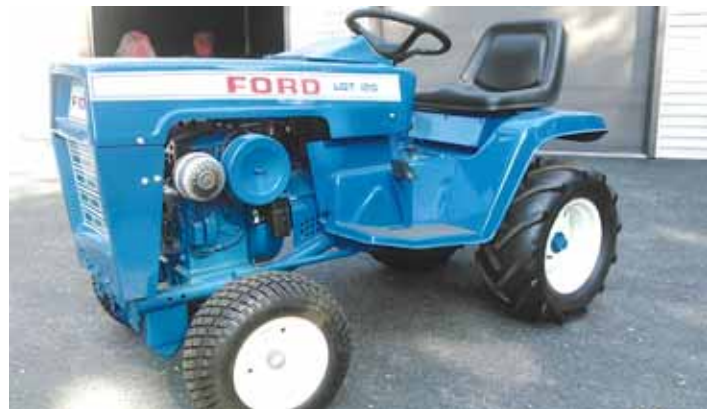
This rare prototype Ford LGT 120 garden tractor was introduced in the early 1970's. "There are several differences between it and the production model," says owner Josh Deaven.
