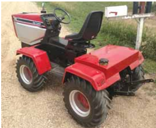
Starting with the frame of an 1864 Cub Cadet, Harold Dejong built this 4-WD tractor that looks like a miniature version of an IH 5088.
