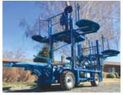
As automated harvester moves through the field, an "air knife" pushes picked berries As automated narvester moves through the rely, an an kinner pushes picket berries onto a conveyor which delivers them into a collecting bin. Photo at right shows the company's self propelled picking machine with hydraulically-controlled platforms.
