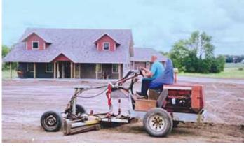
Self-propelled rake uses a 9-ft, wide rotating drum to chew up the soil and shove small rocks off to the side, leaving a smooth seedbed to plant grass into.
