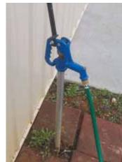
A 2-ft. long pipe mounted on hydrant handle provides operator with more
