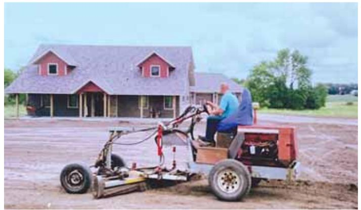
**Self-propelled rake uses a 9-ft. wide rotating drum to chew up the soil and shove small rocks off to the side, leaving a smooth seedbed to plant grass into.**
