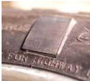
two issues ago, FARM SHOW featured a company called **Glue Tread** that sells a kit for fixing cuts on tractor tire sidewalls. I had several severe cracks and splits up to 4 in. long on a tractor. So I called and was delighted at the 2-day turnaround. Since I applied the strips to the tires, I've pulled a heavy disk for 8 to 10 hrs. and baled 160 bales and everything seems fine so far ([www.GlueTread.com](http://www.GlueTread.com); 800 238-9791).
