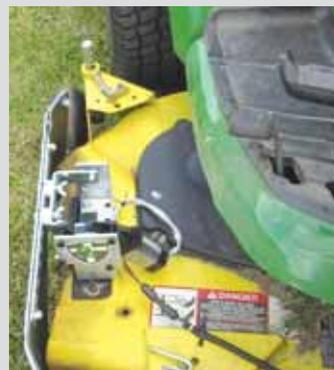
Motorized rubber guard opens and closes over mower chute opening. To operate the guard on his garden tractor, Streib made a pvc mounting bracket and mounted a toggle switch on it.
