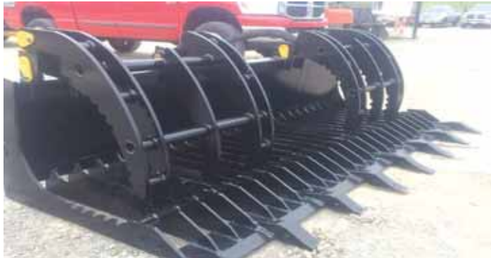
Rance Bryan's quick-tach rock grapple comes with 2 grapple arms independent from one another. Works great when handling uneven loads.
