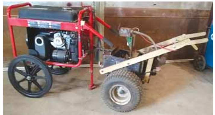
Johnson mounted an electric motor on the transaxle off a riding mower. Motor is wired to generator and used to belt-drive the transaxle. A pin serves as a pivot point that makes the generator easy to steer.
