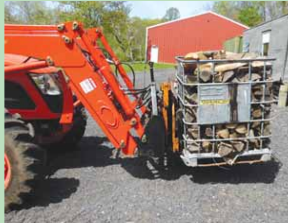
"Rotating forks" let Petrevich lift steel totes loaded with firewood over the side of a dump truck, then rotate them upside down to dump wood directly into truck.
