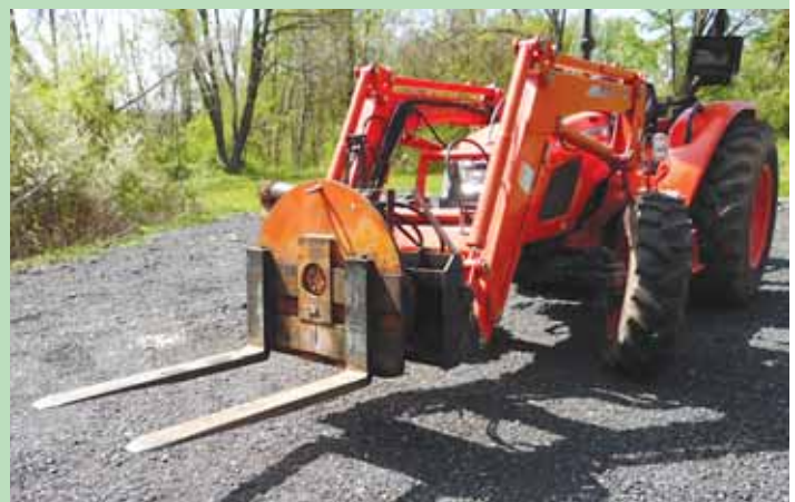
Extending a hydraulic cylinder causes semi-circular steel plate and forks to rotate 180 degrees.
