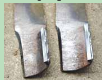
Welded-on key stock creates additional turbulence inside deck to keep grass flowing.
