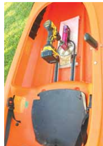
Slate powered his kayak using the bottom gearbox and propeller off an outboard motor, a bicycle gear, and a cordless drill. Garage door opener chain runs from gear to back of kayak.
