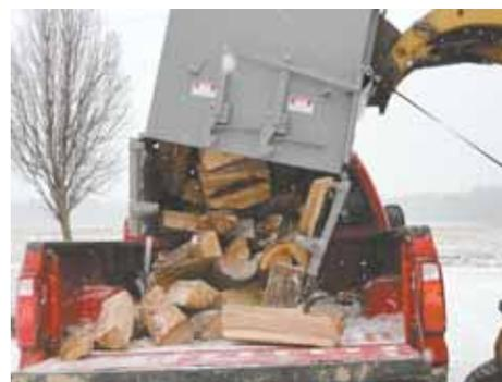
Bottom-unloading hopper lets you load firewood into a pickup or trailer bed without worrying about damaging the vehicle. Hopper slowly empties as it's raised.
