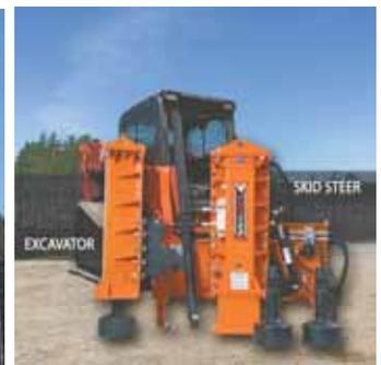
Eterra recently introduced this new skid steer-mounted post driver that doubles as a concrete buster. It can be fitted with multiple heads and fits any loader, as shown above.
