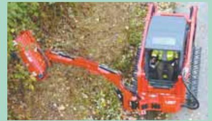
The Raptor Boom Mower for Skid Steer Loaders (left) is ideal for roadside vegetation clearing, trail maintenance, property landscaping, park maintenance and more. The Raptor system can also be fitted with a Flail Mower (above) and a Cyclone Rotary Cutter head.
