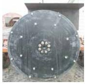
Metal fender over flywheel helps keep dirt from flying up onto tractor.
