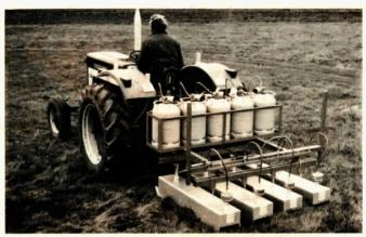
"Ovens" can be spaced for weed control in row crops, or ganged for "broadcast" weed control.
