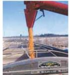
Spring-loaded spout can be adjusted forward or backward by cranking a hand-operated winch at bottom of auger.
