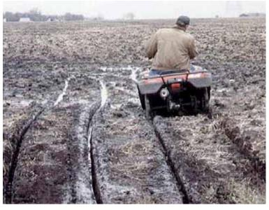
Wheels make a 4 to 14-in. deep trench in muddy ground. Deeper trenches can be made by making repeated passes in the same tracks. Works great for draining water away from flooded fields.
