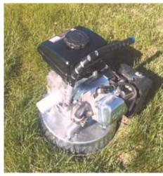
"Predator Gopher Killer" uses a 3 hp., 4-cycle gas engine mounted above an inverted steel pan to kill rodents with carbon monoxide.
