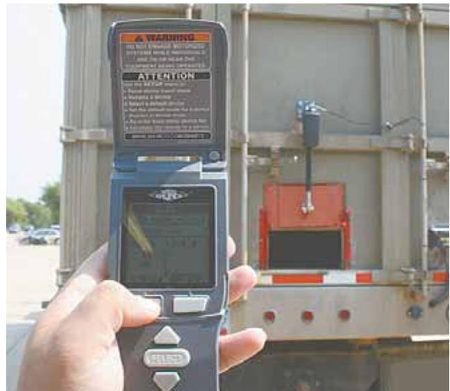
tric tarp, a smart wire system allows plug-and-play operation. The tarp, gate and hoist can be controlled by the same mini-module, and other electronic accessories such as an electric hopper opener, an electric swingaway, and work light packages can also be added. Depending on the products used the installation will take anywhere from a few hours to a day.
